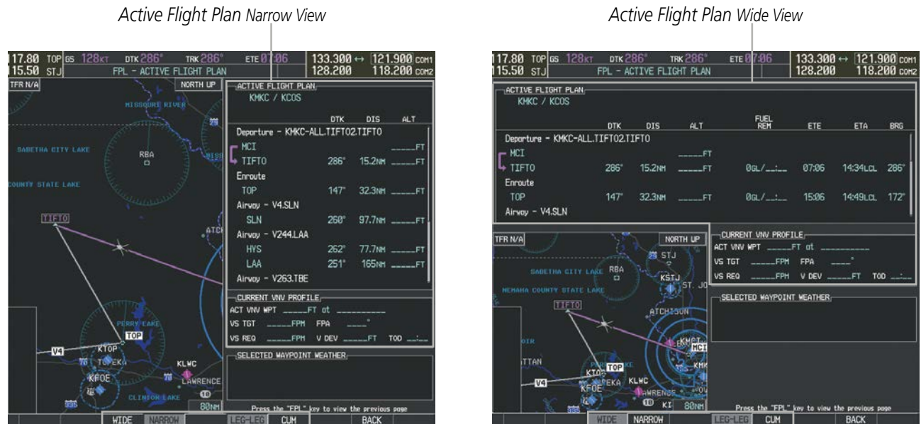
Figure 5-87 Active Flight Plan - Wide vs. Narrow View
