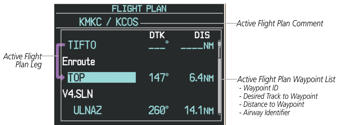
Figure 5-57 Active Flight Plan Window on PFD
