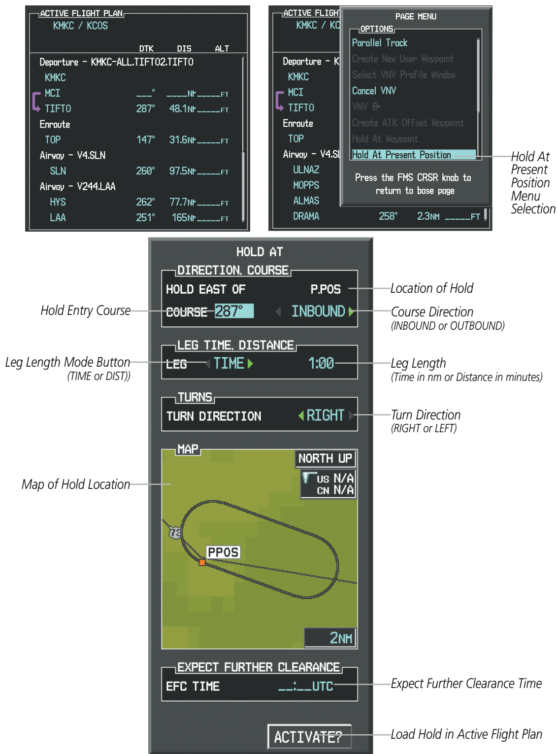
Figure 5-90 Creating a User Defined Holding Pattern at the Aircraft Present Position
