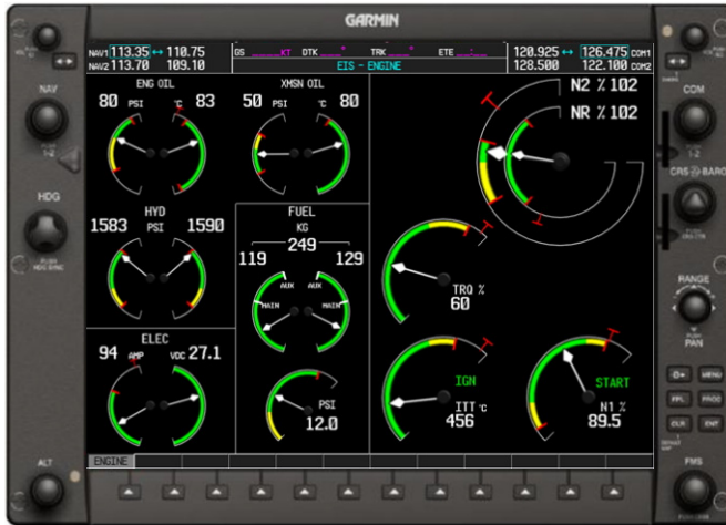
Figure 7-12. Representative Start/Auto Mode Display for G1000H (for reference only)
