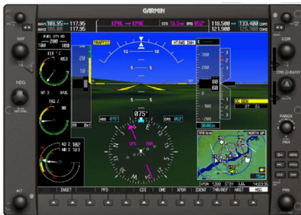
Figure 7-8. PFD with 360° HSI depicts basic PFD functionality (shown with SVT) (for reference only)
