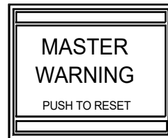
RED MASTER WARNING LIGHT (MWL)
