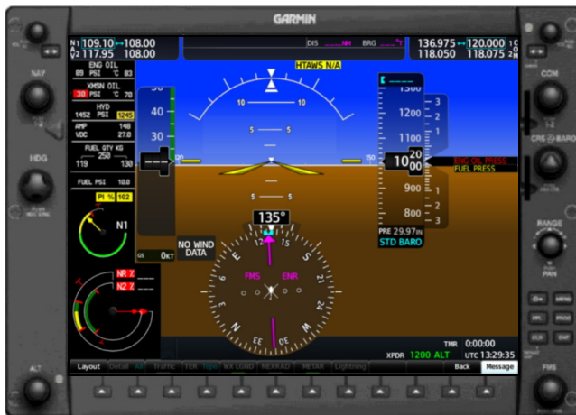
Figure 7-14A. G1000H NXi Primary Flight Display (PFD) with Inset Display of EIS (for reference only)
