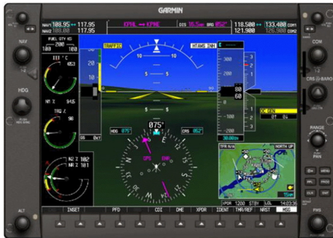
Figure 7-11. Representative Reversionary Mode Display for G1000H (shown with SVT) (for reference only)
