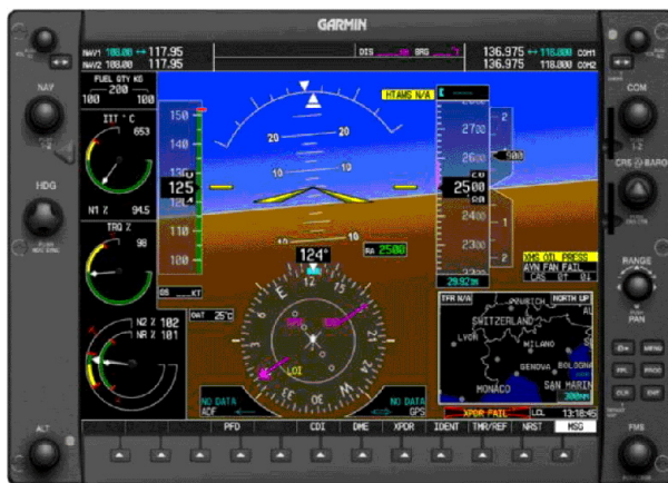
Figure 7-6. G1000H Primary Flight Display (PFD) with Inset Display of EIS (for reference only)
