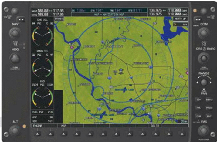
Figure 7-10. Representative Normal Mode Display for G1000H (for reference only)
