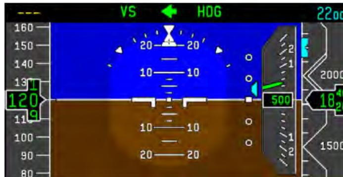
3. The AW139 does not have a separate Turn Co-ordinator. When flying manually, turn coordination is maintained as part of the Yaw Control function which engages automatically when either autopilot is engaged and when ATT or SAS mode are active. When coupled, the Flight Director will automatically produce a Rate 1 or Standard Turn. However, when flying manually, the pilot will have to determine the angle of bank appropriate to the selected airspeed.
